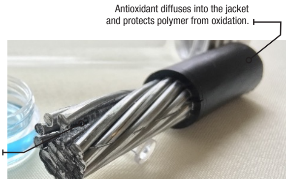
Fig. 3. Silicone gel is a unique two-part material that transforms from a easy-flowing mixture into a non-flowable gel in approximately 48 hours.
