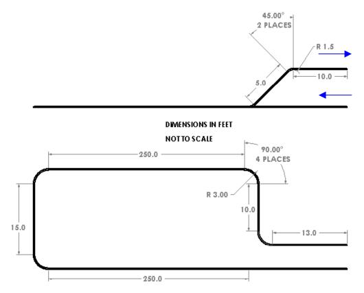
Figure 1: Approximate Layout of Conduit Run
