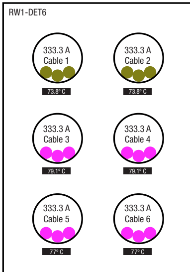
Graph 1 - Underground Duct Bank, Direct Buried in Soil
