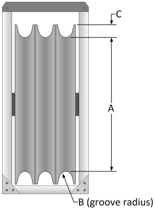
Figure 4: Measurements for stringing sheave.
