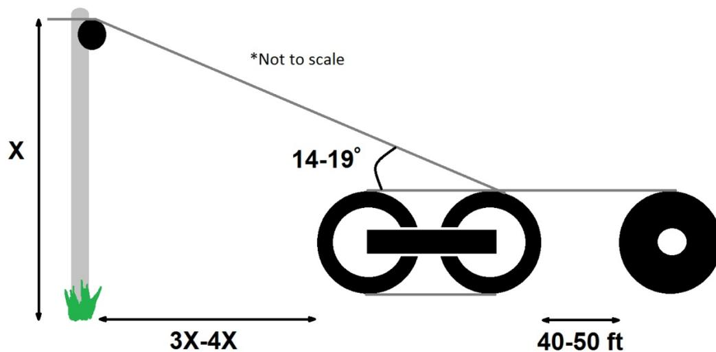
Figure 3: Orientation for bullwheel/payoff setup.
