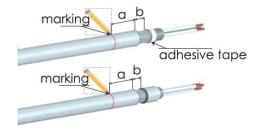
3. Insert cable into cable gland until marking "a" aligns with cap.
