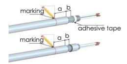
3. Insert cable into cable gland until marking "a" aligns with cap. EMC component will contact shielding.
