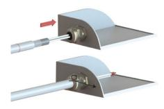
**4.** Do not pull or rotate cable after insertion. In doing so, cable gland and shielding will be damaged.
