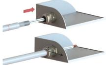
**4.** Do not pull or rotate cable after insertion if no adhesive copper tape is used (2b). Otherwise, cable gland and shielding could be damaged.
