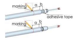
**3.** Insert cable into conductive cable gland until marking "a" aligns with cap.
