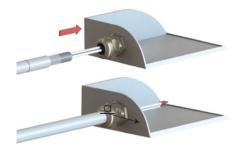
**4.** As long as the cap is not tightened, you can easily pull, push, or rotate the cable.
