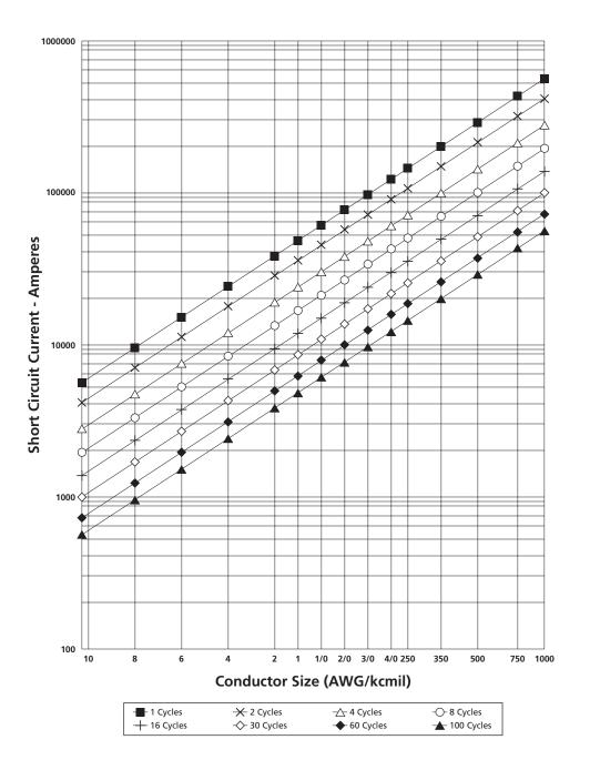
Figure 6-17 Allowable Short Circuit Currents for Thermoplastic Insulated Copper Conductors Rated 105°C Maximum Continuous Operation
