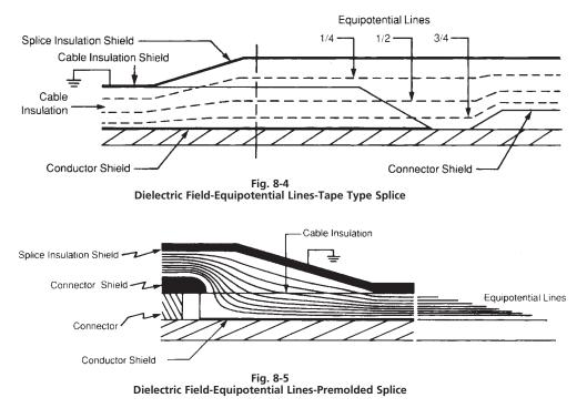
In the preceding figures, the representations of the dielectric fields neglect the differences between the dielectric constants of the cable dielectric and the splice materials.
