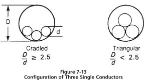
A cradled configuration develops when three single-conductor cables are pulled into a conduit where the D/d ratio is 2.5 or greater. A triangular configuration develops when three single conductor cables are pulled into a conduit where the D/d ratio is less than 2.5. These cables may be pulled from individual reels, tandem reels, or a single reel with parallel wound cables.
