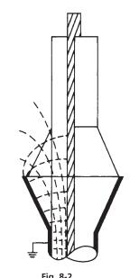
Fig. 8-2 Dielectric Field - Receding Ground Plane - Stress Relief Cone
