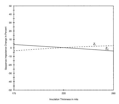
Figure 6-23 Effect of Insulation Thickness on Sequence Impedance
