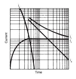
Figure 9-1 Components of DC Test Output Current
