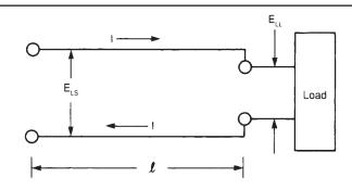
Figure 6-3 AC Single-Phase, Two-Wire Circuit
