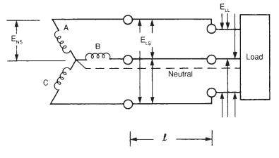
Figure 6-4 AC Three-Phase, Y (Wye) Circuit
