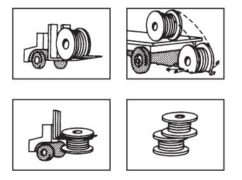
Figure 7-8 Improper Reel Handling
