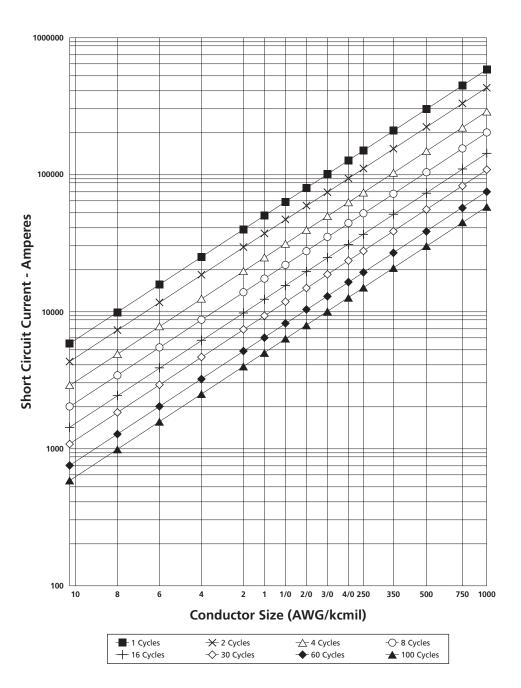
Figure 6-16 Allowable Short Circuit Currents for Thermoplastic Insulated Copper Conductors Rated 90°C Maximum Continuous Operation
