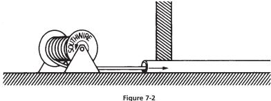
Figure 7-2 Cable Feed into Conduit at Floor Level
