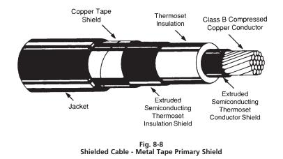
Observe the additional components in comparison to the nonshielded cable. The metallic shielding may be tape instead of wire.
