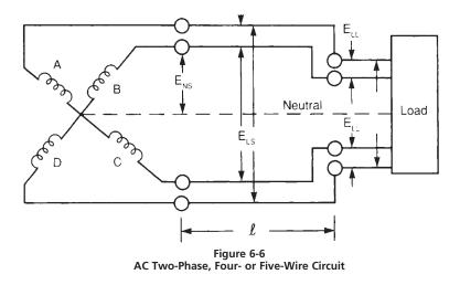
These four- or five-wire circuits are variations of the three-phase circuits previously discussed. Typically, the armature windings and resulting outputs are 90 degrees apart. Other configurations can include three-wire, two-phase; four-wire, two-phase; and four-wire with two isolated phases. Eliminating winding A and D in Figure 6-6 would illustrate a three-wire, two-phase circuit.
