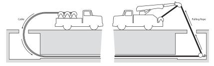
Figure 7-1 Pulling Cable in Duct
