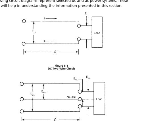
The following circuit diagrams represent selected dc and ac power systems. These diagrams will help in understanding the information presented in this section.
