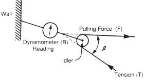
Figure 7-11 Variables for Dynamometer Correction Equation
