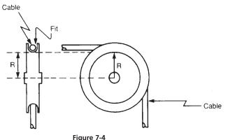
Figure 7-4 Single Sheave for 90° Change of Direction (R is radius used to calculate sidewall pressure, SP)
