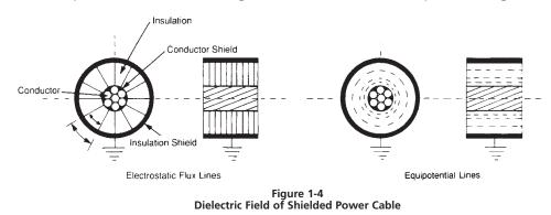
In a shielded cable, all the voltage difference between the conductor and electrical ground is contained within the cable. For nonshielded cable, the voltage difference between conductor and electrical ground is divided between the cable dielectric and any intervening air or other materials.
