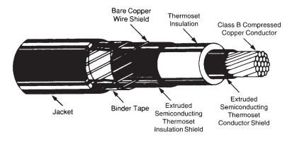
Fig. 8-7 Shielded Cable - Wire Primary Shield
