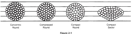
Figure 2-1 Comparative Sizes and Shapes of 61 Strand Conductors
