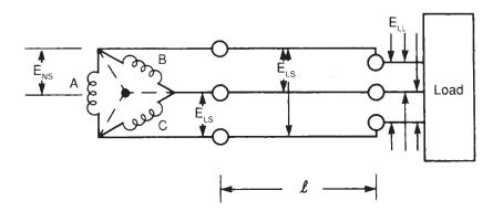
Figure 6-5 AC Three-Phase,  $\Delta$  (Delta) Circuit
