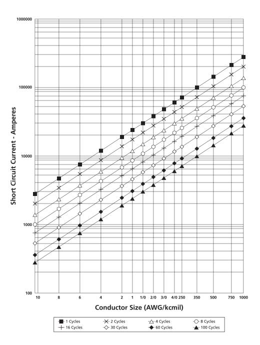
Figure 6-18 Allowable Short Circuit Currents for Thermoplastic Insulated Copper Conductors Rated 75°C Maximum Continuous Operation
