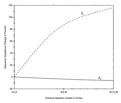
Figure 6-24 Effect of Cable Spacing on Sequence Impedance
