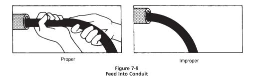
j. Do not pull cable directly across short, sharp angles. After pulling completely out of one side of the enclosure, feed cable into the other side of the enclosure and pull that segment.
