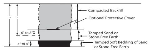
Figure 7-18 Typical Burial Cross-Section TABLE 7-10
