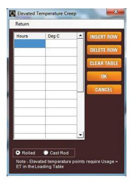
Enter the total time for which the conductor is expected to experience elevated temperatures over the life of the line. Entries are in hours and °C.
