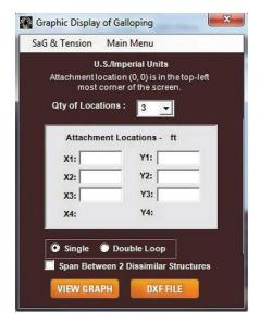
To display a graphical layout of the galloping ellipses, you will need to enter two- dimensional Cartesian coordinates for conductor attachment points. Click on the arrow to the right of the **Oty of Locations** box to select a display of 1 to 4 conductors. An equal number of pairs of attachment point boxes will be displayed, (X1,Y1) thru (X4,Y4).
