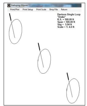
You can print or plot this image directly, or transfer it to a graphics program for further customizing, such as adding to or removing part of the image, setting margins, and/or rescaling before printing/plotting.
