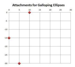
Above is a plot of the following attachment locations: (0,-15) (5,-30) (10,0). This layout is typical for a 3-phase system on a single pole davit arm or post insulator.
