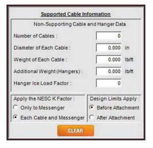
**Hanger Ice Load Factor** is a factor added to account for ice buildup on the hangers. Determination of the amount of ice is left to the design engineer. The number that has traditionally been used, based on 0.50 inches of ice buildup on the hanger, is a value of 1.8. Southwire does not endorse or recommend this number. For other ice buildup thicknesses, enter your calculated value.
