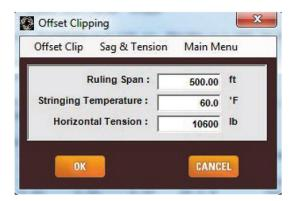
The most recently calculated Ruling Span is displayed as the first input. If you choose that Ruling Span and a stringing temperature from the most recent Sag and Tension run, then the correct Horizontal Tension will be offered as the third input.
