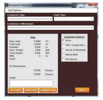
The **Conductor Selection** screen has five main components:
