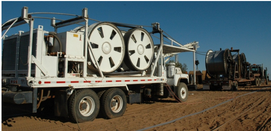
Figure 7. Dual drum bullwheel, courtesy of Oncor.
