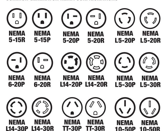
When considering what generator cables and adapters you need for a project, you want to avoid voltage drop from the generator. To do this, utilize as short a cable as possible, along with the largest conductor (smallest AWG) and a connector with as high amperage and voltage rating possible. For instance, you will get less power and greater voltage drop out of a generator using a 100' 15 amp 12/3 extension cord with 5-15 plugs compared to a 50' 20 amp 10/3 extension cord with a 5-20 plug.
